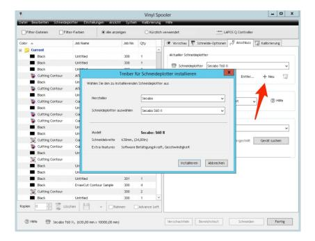
Click on the button labeled "Search device" and follow the instructions in the installation wizard. Confirm the message regarding successful installation by simply clicking on the button labeled "Done". Now you can control your ESC60 stencil cutter using DrawCut.
