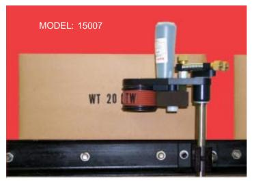
MARSH'S® Reservoir Ink Cartridges plug right into the Mini-Coder for convenient, automatic re-inking of the ink roll during production. Standard models are supplied with MARSH'S® Ribtype die fastening system, a dry Microcell ink roll and an anodized aluminum mounting bracket.
