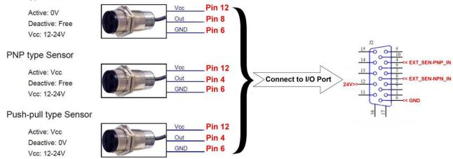
Connect sensor to machine using external power supply. Below demonstration is for external power supply of 5VDC.
