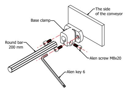
Step 3 Installing the clamps to the round bar.
