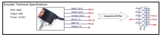
To calculate wheel diameter (**D**) depend on resolution (**R**) is: **D** = **R**/( $\pi$  x 600) (inches).
