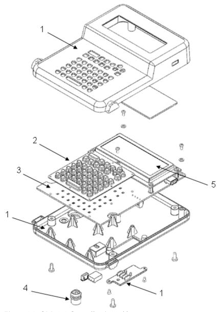
Figure 6-3: QM1610 Controller Assembly
