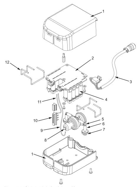
Figure 6-2: QM1610 Printhead Assembly
