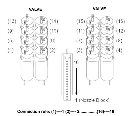
Figure 5-1: Printhead PCBA to Nozzle Block Diagram
